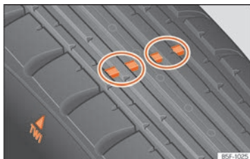
Fig. 277 Tyre profile: tread wear indicators.
