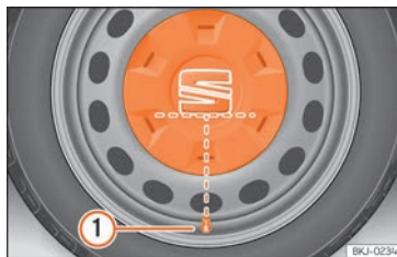
Fig. 34 Correct positioning of the central wheel trim for steel rims.
