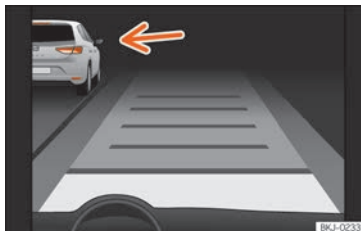
Fig. 238 On the instrument panel display: ACC active, vehicle detected in an outer lane.
