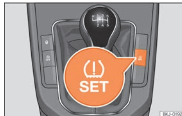
Fig. 279 Centre console: tyre pressure loss indicator button.
