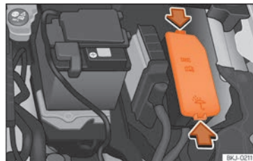
Fig. 52 In the engine compartment: fuse box cover.
