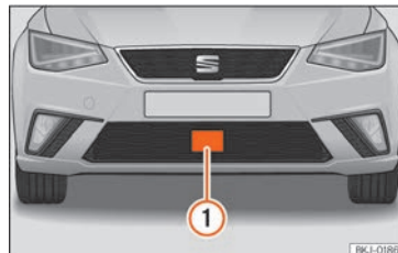
Fig. 235 On the front bumper: radar sensors.
