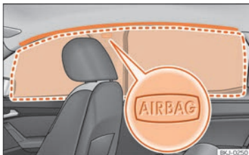
Fig. 21 Location and deployment area of the head-protection airbag.
