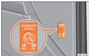
Fig. 17 Switch for activating and deactivating the front passenger airbag.
