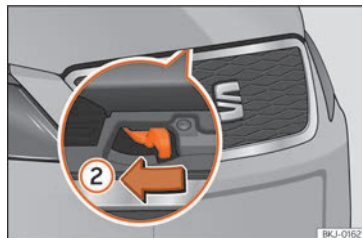
Fig. 268 Lever under the bonnet.
