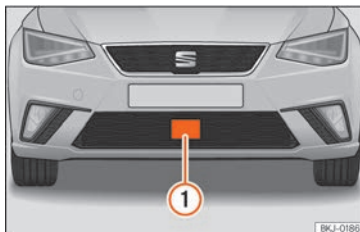
Fig. 229 On the front bumper: radar sensors.
