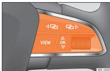
Fig. 78 Right side of the multifunction steering wheel: buttons to the menus and information displays on the instrument panel.
