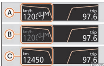
Fig. 225 On the instrument panel display: indications of the speed limited status.
