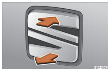
Fig. 99 Rear lid: opening from outside.
