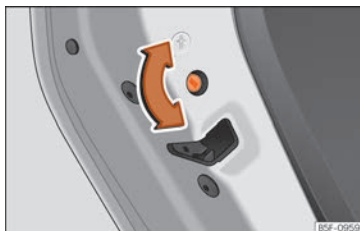
Fig. 98 Childproof lock on the left hand side door.
