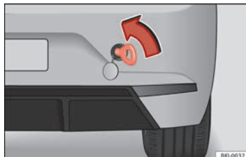
Fig. 108 Right side of the rear bumper: towline anchorage screwed in.
