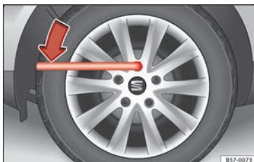
Fig. 81 Changing a wheel: loosen the wheel bolts.
