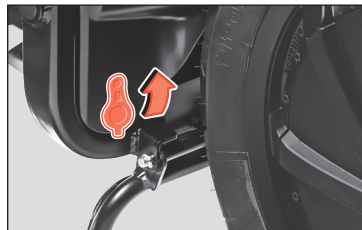
Fig. 1 Left side of the eScooter: safety latch
