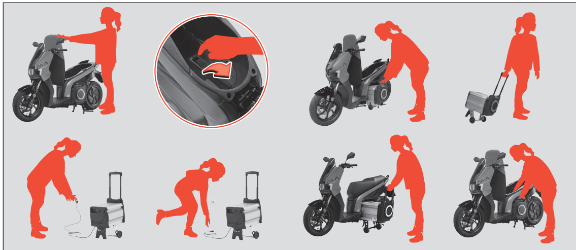
Fig. 31 Removing the battery
